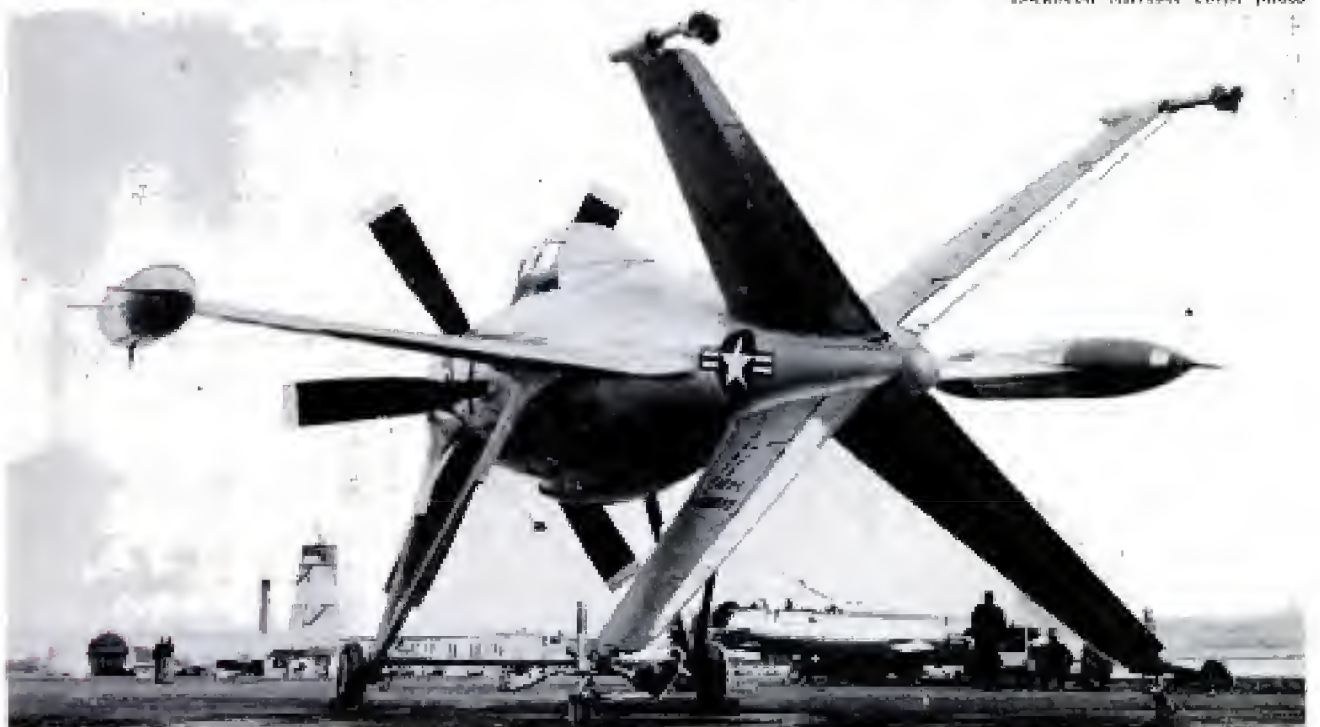
High, old-style landing gear will be used on the XFV-1 during its first test flights and then discarded
